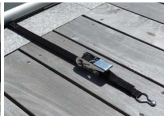
Adjustable straps with stainless-steel ratchets
